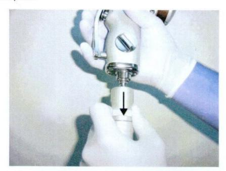
Slide quick-disconnect outer-shell in direction shown to secure hose to the Woodpecker.
